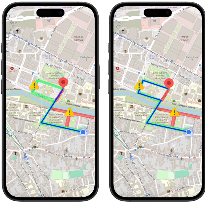
Fig. 4. Mobile application interface for PoC#2 illustrating routes conditions. The left screen shows the optimal route from a distance perspective (minimum distance), while the right screen presents the most accessible route. In both views, the route quality is color-coded (e.g., red for mobility-related problems, green for no issues), alert markers highlight specific obstacles such as steep slopes or temporary barriers.
